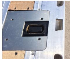
**Fontaine twist locks** are placed behind the siderail to help protect the mechanism. This stronger design also gives you full use of the siderail load securement system so you can handle conventional loads with ease.
