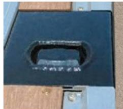
**Competitive twist locks** are cut into the side rail and are exposed to side impact damage from fork lifts. This weaker design interrupts the stake pockets/load securement system and annoys drivers.
