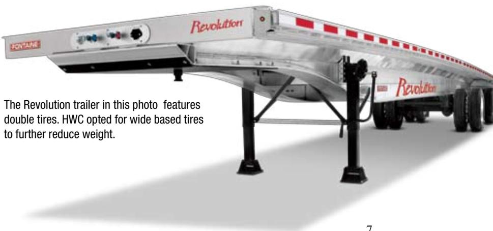
The Revolution trailer in this photo features double tires. HWC opted for wide based tires to further reduce weight.
